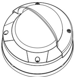
This manual is intended for users of the DA-SS1100 sun shield. It includes instructions for mounting the DA-SS1100 sun shield to the camera body.
