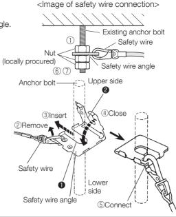
· When the existing anchor bolt that has been installed is used for connecting the safety wire, the use of 2 spacer nuts is helpful.
