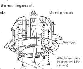
Fixing screw for attachment plate (4 pcs.) (M4: accessory)
