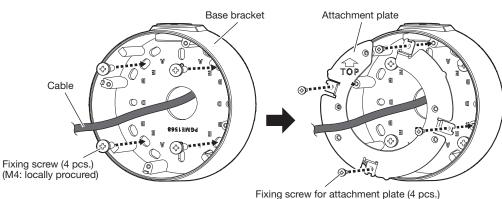
Fixing screw for attachment plate (4 pcs.) (M3×10 mm {13/32 inches}: accessory)
